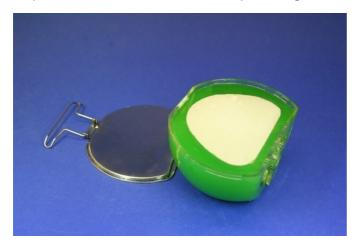
10) Mix the casting resin according to the manufacturer's instructions. Pour a thin stream of resin into the flask through the middle channel until it emerges from the two other channels. Finally, place the flask into a pressure pot filled with water heated to 45 °C for around 25 minutes at 2.5 bar.
