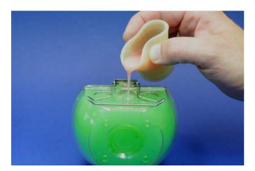
Important: The resin-filled channels must not be immersed in water while the resin is still molten.
