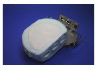
9) Mix the casting resin according to the manufacturer's instructions. Pour a thin stream of resin into the flask through the middle channel until it emerges from the two other channels. Finally, place the flask into a pressure pot filled with water heated to 45 °C for around 25 minutes at 2.5 bar.
